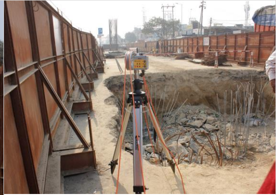
All In One KIT MCHA Ultrasonic Cross-hole Testing Equipment
