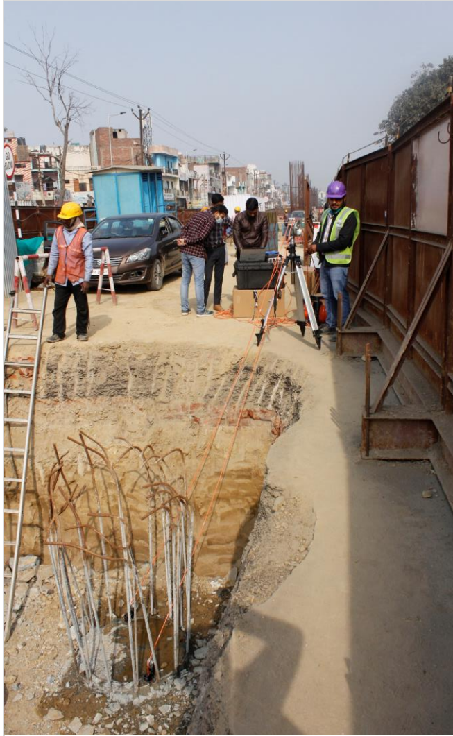
Inserting two probes ( 1 Tx & 1 Rx ) through the pile between two similar water filled tubes.
