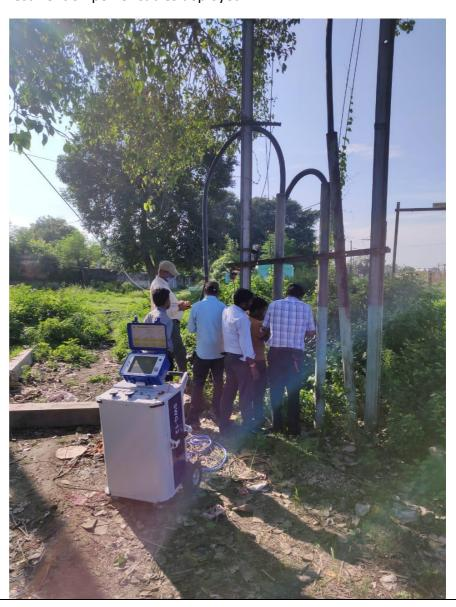
The SWG12 provides 3 surge voltage ranges of 3, 6 and 12 kV respectively allowing the lowest voltage to be applied to the cable depending on voltage breakdown detected.
