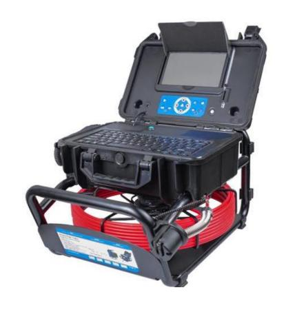
The RPIC2 **Video Pipe Inspection camera** is based on fiberglass semi flexible rod with diameter 6.8 mm & with camera head 23 mm (diameter), in order to inspect high pressure corrugated steel pipe with internal diameter approx. 68 mm, a standard 46 mm skid (a part of kit) was used to centralise the camera head & slip over the corrugation.
