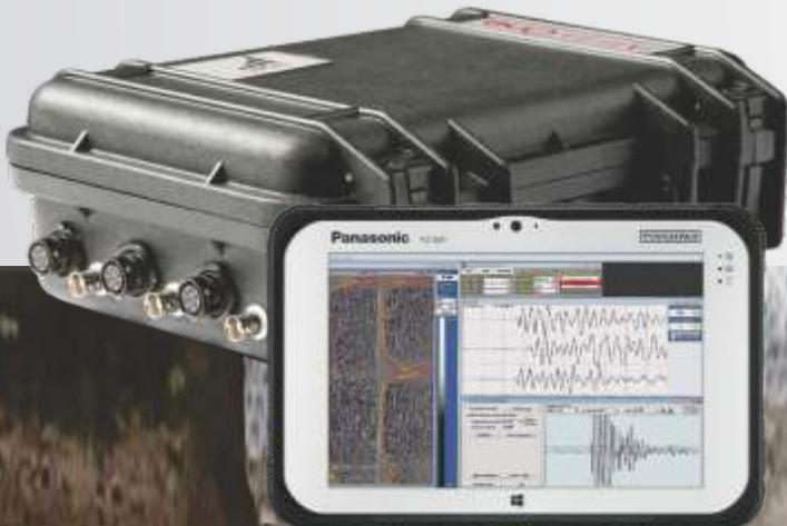
All-in One is a highly ruggedized modular Ultrasonic test kit system that can be configured for checking homogeneity of concrete structures, piles & diaphragms foundation. The instrument is designed for construction, building and geophysical research industry and is available in following configuration options which are future upgradeable for performing the below tests:
