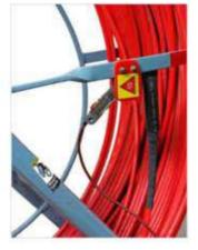
Step 3: Energise the traceable duct rodder with any frequency such as 8/16/33/64/65/133 kHz etc using any signal excitor/ transmitter
