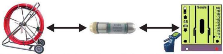
At this point, switch to Sonde mode by choosing the frequency of the Sonde in the Receiver. Follow procedure to locate Sonde and the corresponding location of blockage as shown .
