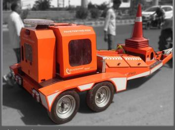
load plate axis. At preset heights, a load is dropped to cause a controlled load pulse in to the ground.
