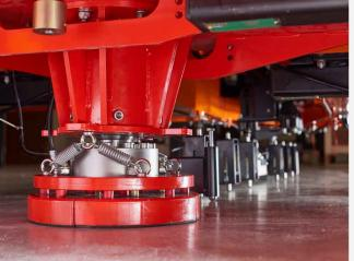
4 way split loading Load cell, 300mm to allow even distribution of load on an uneven surface.
