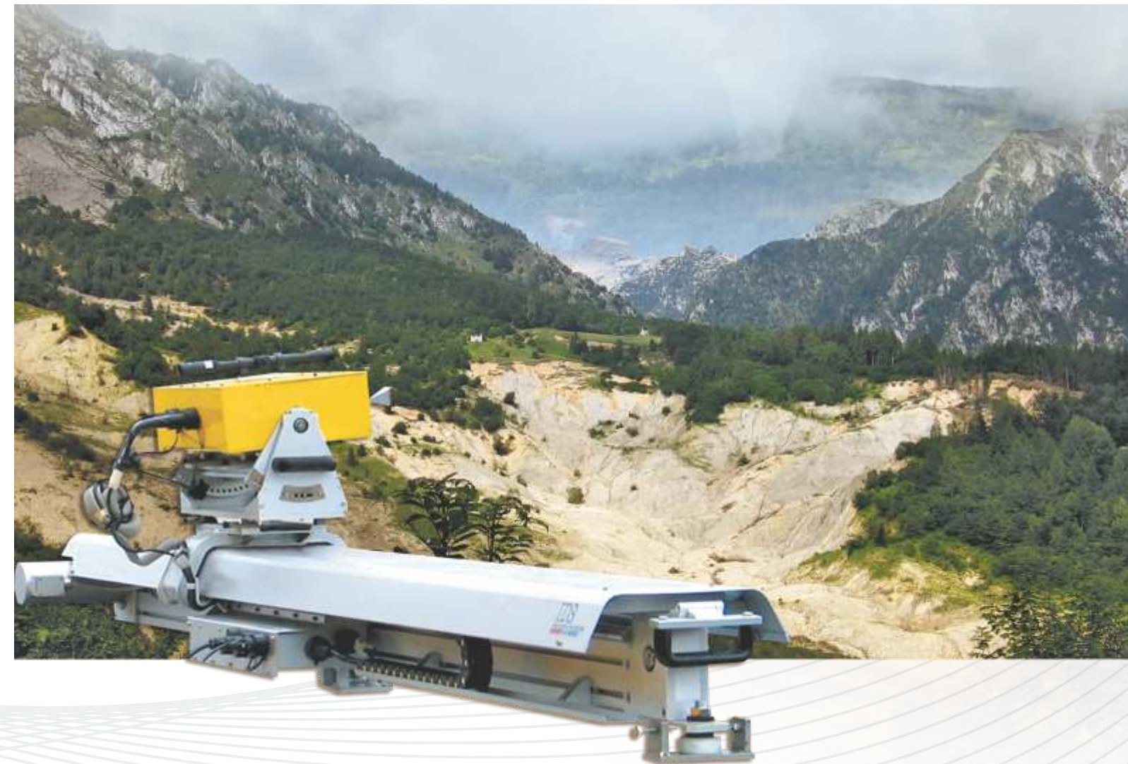
IBIS-FL: REAL TIME REMOTE DISPLACEMENT MONITORING BASED ON MICROWAVE INTERFEROMETRY
