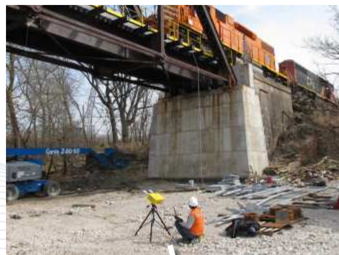
IBIS-FS monitoring an iron bridge
