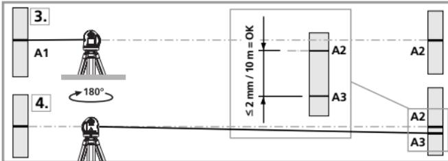
4. Turn the device through 180° and mark point A3. The difference between points A2 and A3 is the tolerance.
