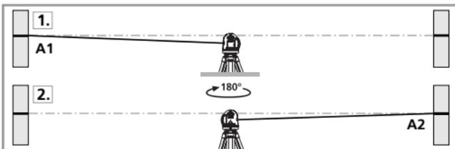
2. Turn the device through 180° and mark point A2. You now have a horizontal reference between points A1 and A2.
