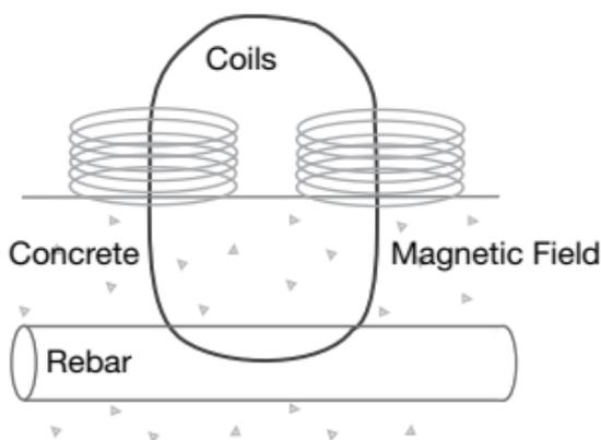
The Profoscope uses different coil arrangements to generate several magnetic fields. Advanced signal processing allows
