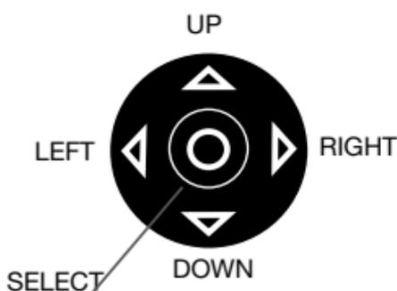
The settings menu can be entered by pressing the select button. Use the navigation keys to select the desired menu icon and press the select button again.
