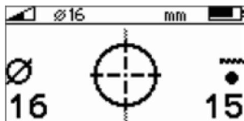
The measured rebar diameter replaces the signal strength arrow.
