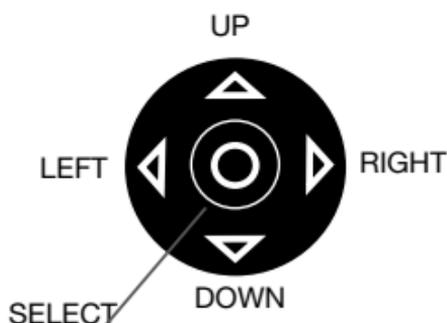
Pressing the up arrow will switch the back-light on/off.
