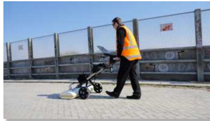
RIS Hi-BrigHT: pavement surveying
