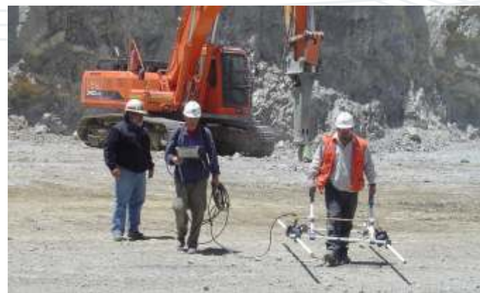
Survey with a low frequency antenna at a mine
