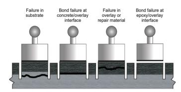
For example "B 100%" indicates a complete failure in the overlay or repair material.
