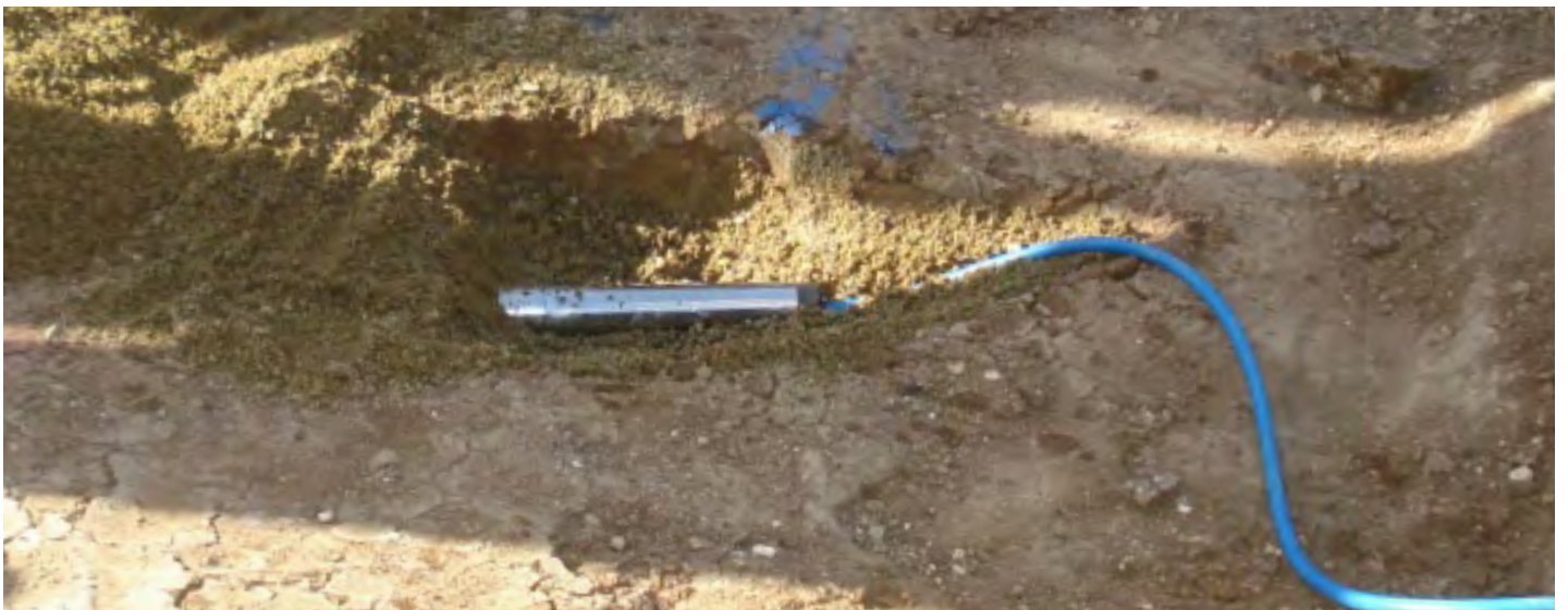
Vibrating wire piezometer in embankment dam foundation
