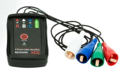
The 3ID Three Phase Cable Identifier is a reliable solution for identifying the correct phases on extended lengths of de-energized and discharged overhead and underground cables. This comprehensive tool consists of both a sender and receiver, designed for easy handling, even with gloves. Each phase or any phase conductors shorted to neutral are clearly indicated with individual lights for quick and accurate identification.
