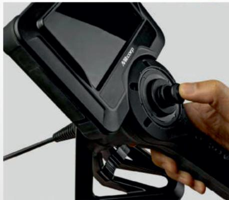
Joystick Control for 360° Probe Operation
