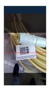
QR code scanner for automatic configuration of analog sensors.
