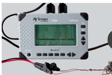
Selecting a Cable & Setting Velocity Propagation (VP)
