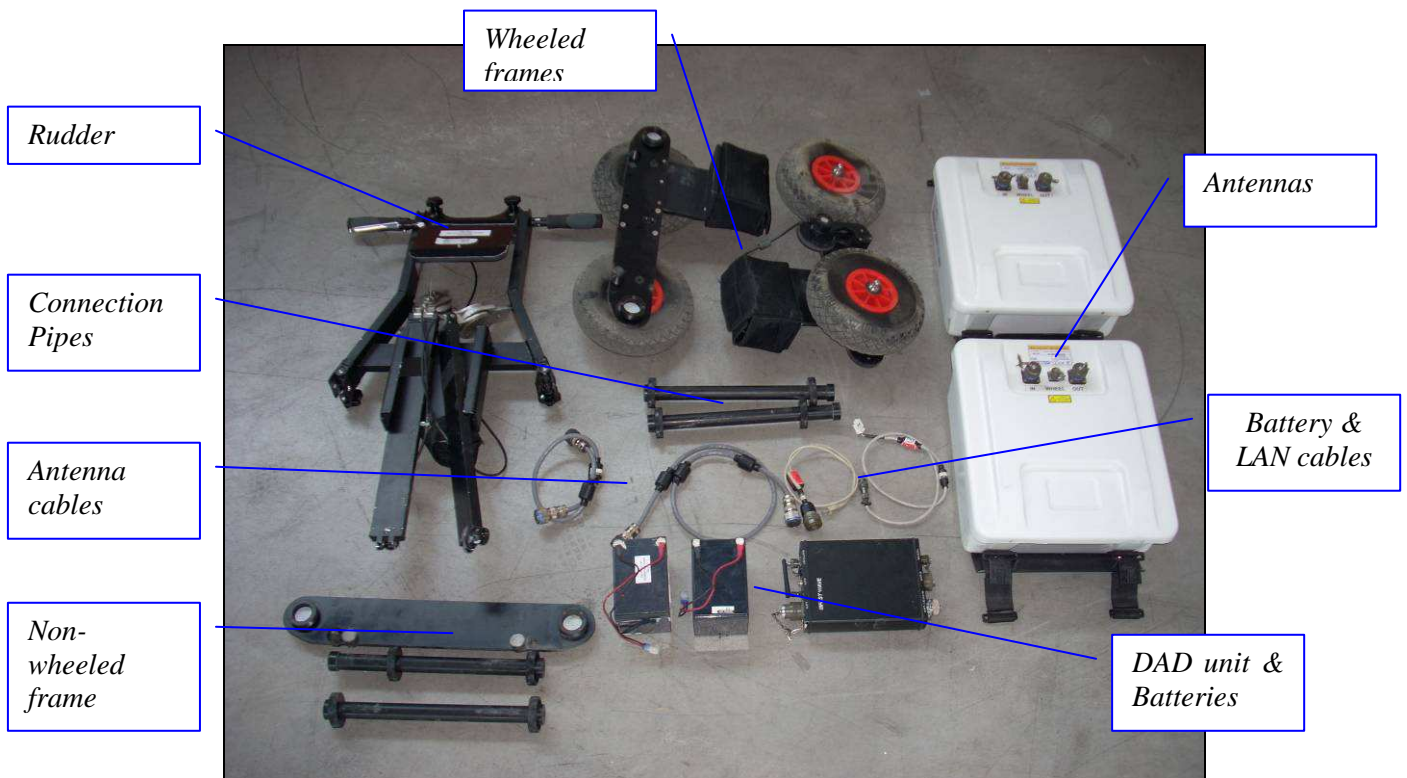
Fig. 1.13 – Equipment provided for the two antennas configuration
