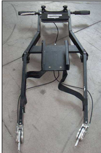
Fig. 1.2 – Rudder in mono antenna configuration
