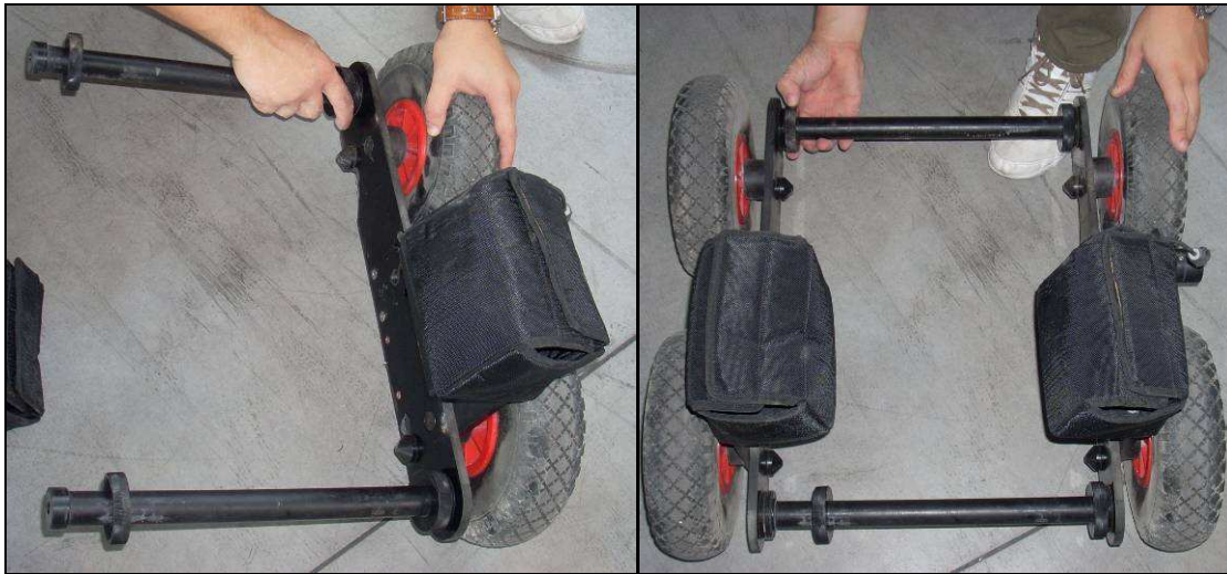
Fig. 1.5 – Connection pipes in position and closed frame
