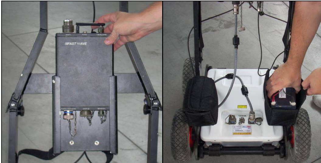
Fig. 1.9 – Insertion of the DAD Control Unit and battery
