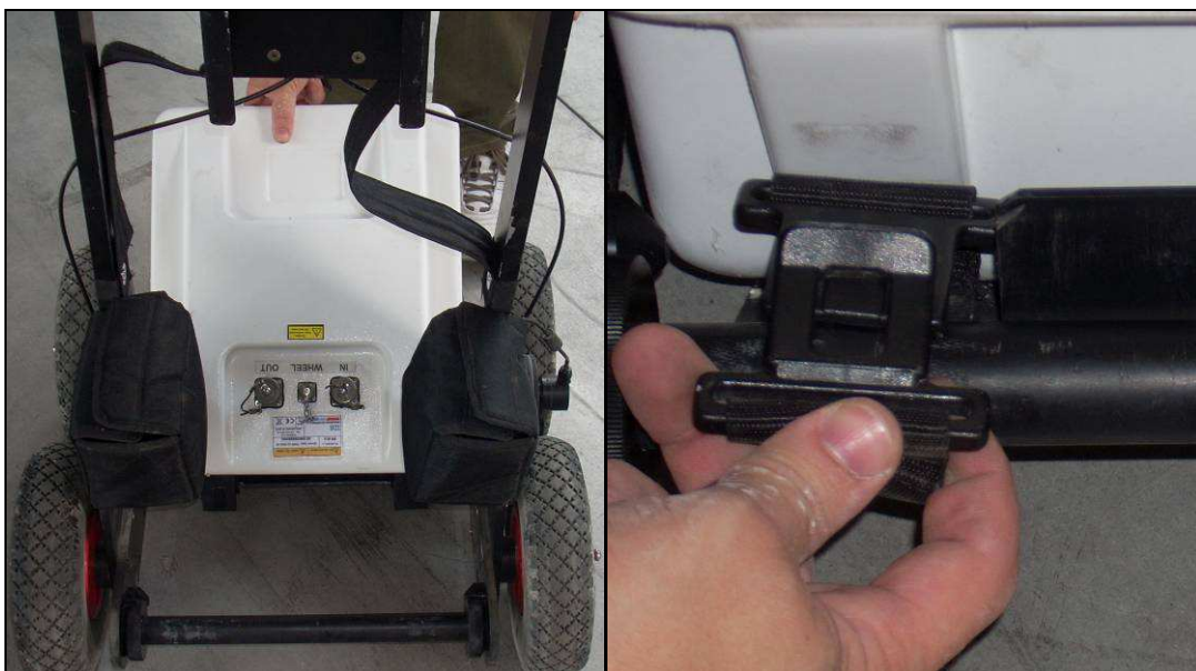
Fig. 1.8 – Insertion of the antenna and close up of the hook
