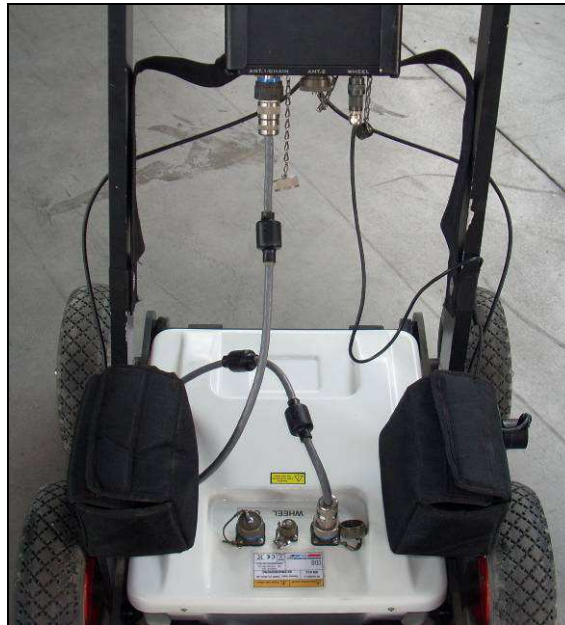
Fig. 1.11 – Antenna cable in place
