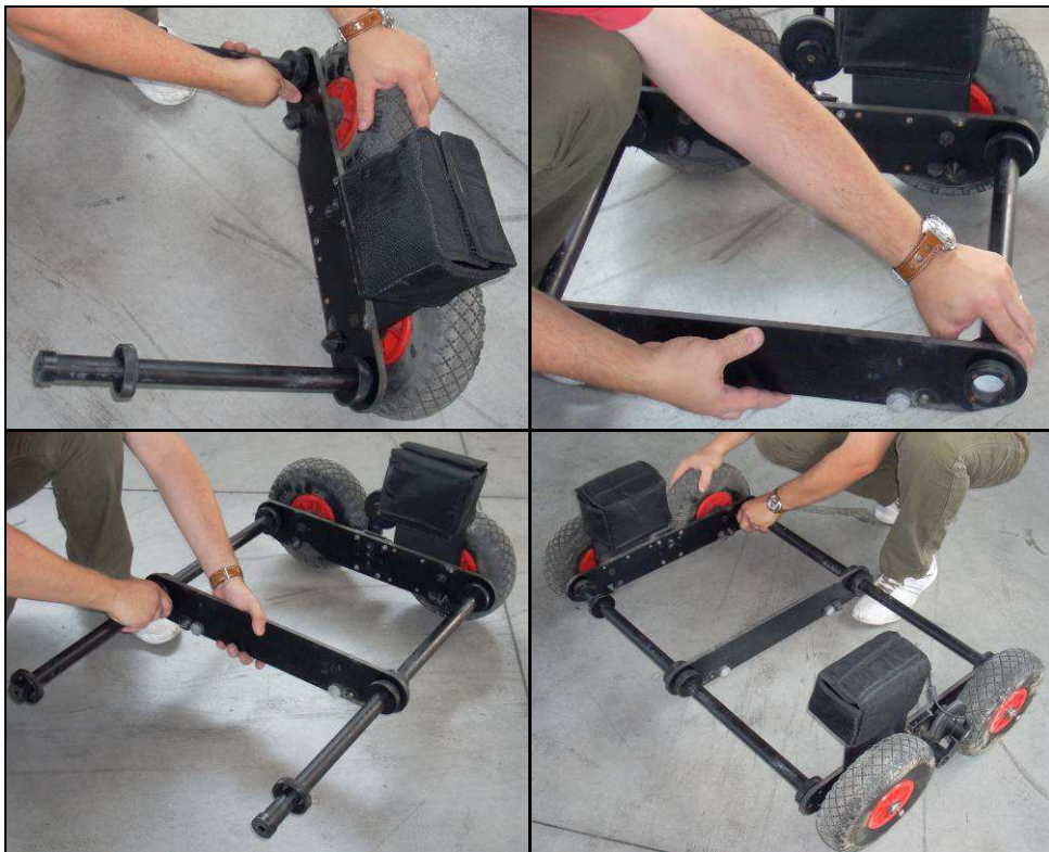
Fig. 1.16 – Making the two antennas frame
