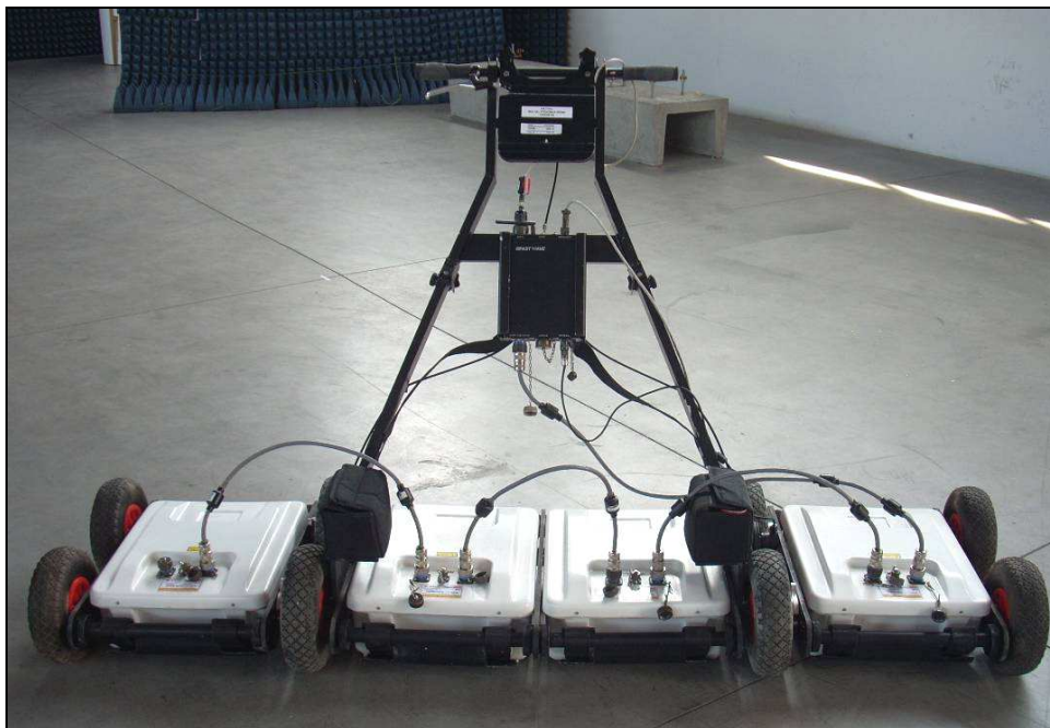
Fig. 1.30 – Four antennas configuration
