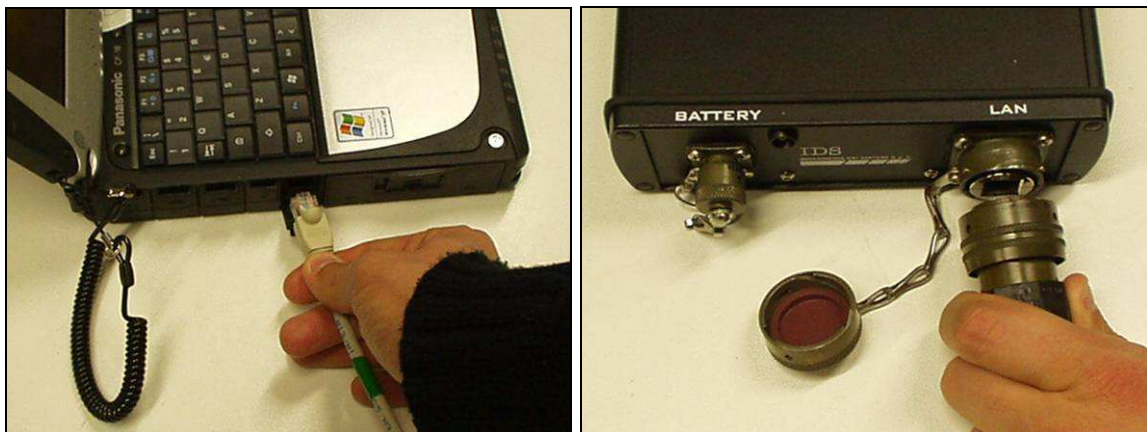
Fig. 2.7 – Lan Cable connection between the Notebook Computer and the DAD Control Unit
