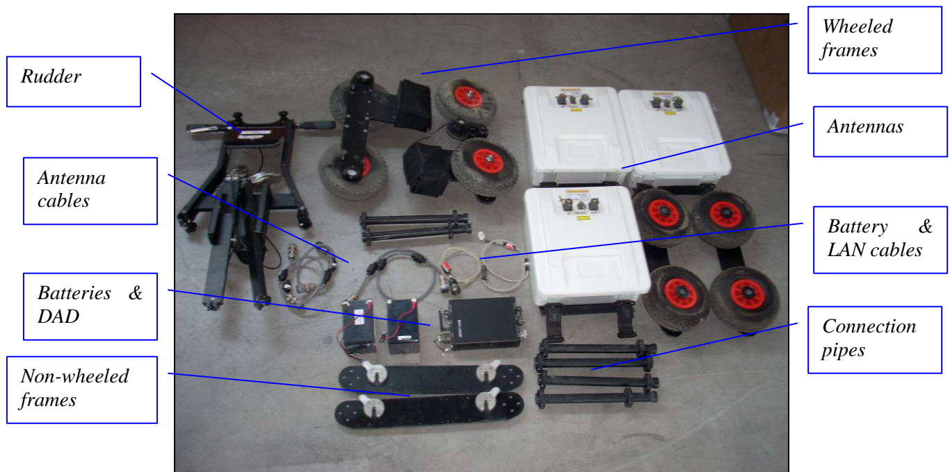
Fig. 1.21 - Equipment provided for the three antennas configuration
