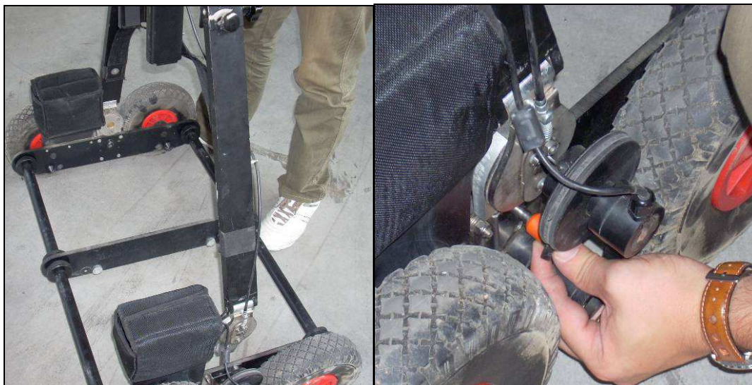
Fig. 1.17 – Insertion and locking of the rudder
