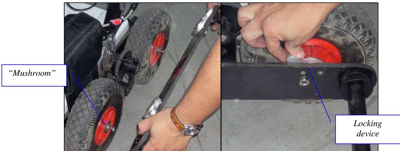
Fig. 1.24 – Main frame “mushrooms” & locking device
