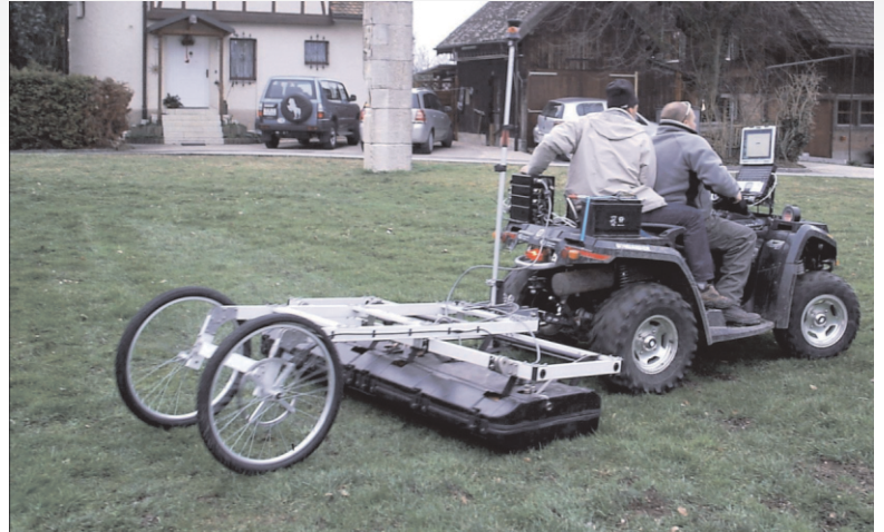
STREAM-X systems : Configure with an array of 200 or 600 MHz antennas.
